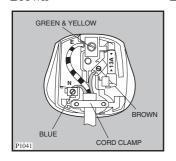
The wire coloured green and yellow must be connected to the terminal marked with the letter  $\ll E \gg$  or by the earth symbol  $\frac{1}{=}$  or coloured green and yellow.
